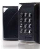
Multi-discipline junction box reader, black, - Dimensions : 12cm x 7.2cm x 1.9cm, - Input voltage 8 - 14 VDC, - Connection type : Wiegand, - Tri-coloured status LED, - Optical tamper protection, - Credential compatibility : Mifare | iClass | HID H1021, H10302 and H10304 | HiTag Impro 125kHz and 13.56MHz slim tag, omega tag, quad transmitter, - Environmental rating : IP20
